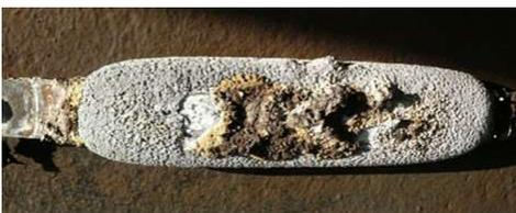
A common way to minimize the corrosive effects on boats is to utilize sacrificial anodes made of zinc, aluminum or magnesium. These anodes preferentially absorb the charges and corrode first, which protects the more valuable metals such as the boat hull or propeller. This can either be passive or induced (with electricity), but the key piece is that these anodes MUST be in the water in
